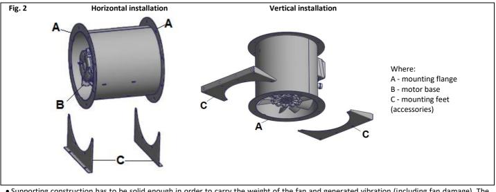
• Supporting construction has to be solid enough in order to carry the weight of the fan and generated vibration (including fan damage). The fan cannot be exposed to vibration.
