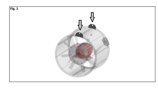
• Do not approach lifted device. In case of breaking, falling device may cause serious injury or death.
