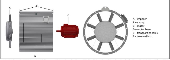
The fan housing (B) is made of sheet steel. The housing is welded and then hot dip galvanized. The impeller blades (A) and the hub are cast from aluminum, while the hub insert is made of steel. Connecting elements made of steel, galvanized steel and stainless steel were used.
